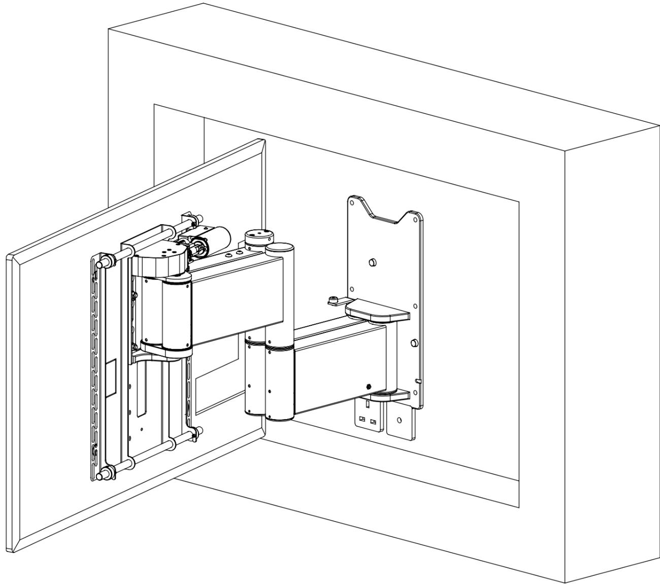
A recess 10mm larger than the perimeter of the screen is acceptable. The screen will move out before turning. Allow for screen ventilation when creating recesses as tight as this.
